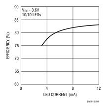
Figure 4. Efficiency vs LED Current, Circuit of Figure 3
