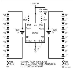
Figure 3. Li-Ion to 10/10 White LEDs
