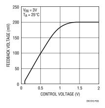
Figure 5. Feedback Voltage vs V<sub>CTRL</sub>
