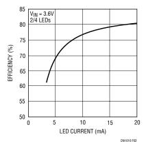
Figure 2. Efficiency vs LED Current, Circuit of Figure 1
