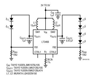
Figure 1. Li-Ion to 2/4 White LEDs
